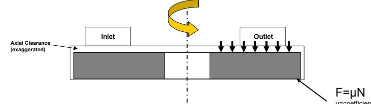
Diagram shows 'single sided' porting arrangement. Rotor set is forced against the housing floor (all axial clearance assumed to be at porting side of housing)
