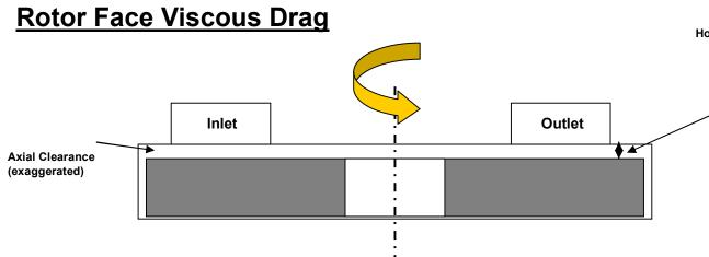
Diagram shows 'single sided' porting arrangement. Rotor set is forced against the housing floor (all axial clearance assumed to be at porting side of housing)
