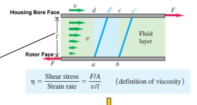
A = Area of rotor faces moving against housing face
