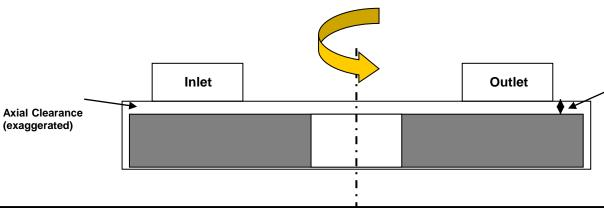
Diagram shows 'single sided' porting arrangement. Rotor set is forced against the housing floor (all axial clearance assumed to be at porting side of housing)
