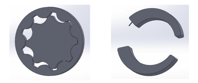
Once the gerotor (and porting if required) geometry is defined, solid CAD models can be output in various formats directly from the software interface.
