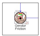
The Gerotor Friction object contains the parameters which affect the dynamic friction of the pump, including axial clearances, face areas, friction torque radii, rotor width and shaft information.
