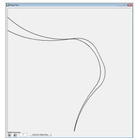
Changes can be made to the parameters of the gerotors at this point, perhaps to see their effect on the geometry or to closer align with an existing gerotor set. Once the porting and performance calculations have been completed, this step can be returned to again to refine the geometry especially regarding contact stress alleviation or efficiency improvements (usually related to clearances).
