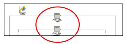
These two leakage objects represent the axial leakage either side of the gerotor set.
