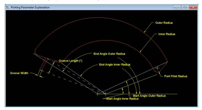
The 'zero' line for the angular dimensions is the horizontal line, to the right of the centreline of the inner rotor (i.e. the 3 o'clock direction on a clock face). Positive angles are measured anticlockwise from this line.
